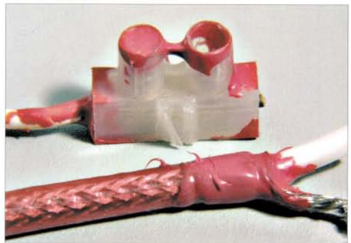
● Fig. 2: Two typical cases where Liquid Electrical Tape would prove useful in any antenna installation.
