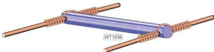
● Fig. 1: Using small lengths of a thinner wire to fix open wire feed spreaders in place. The wires may be left, as shown or soldered in place for slightly more stability.
